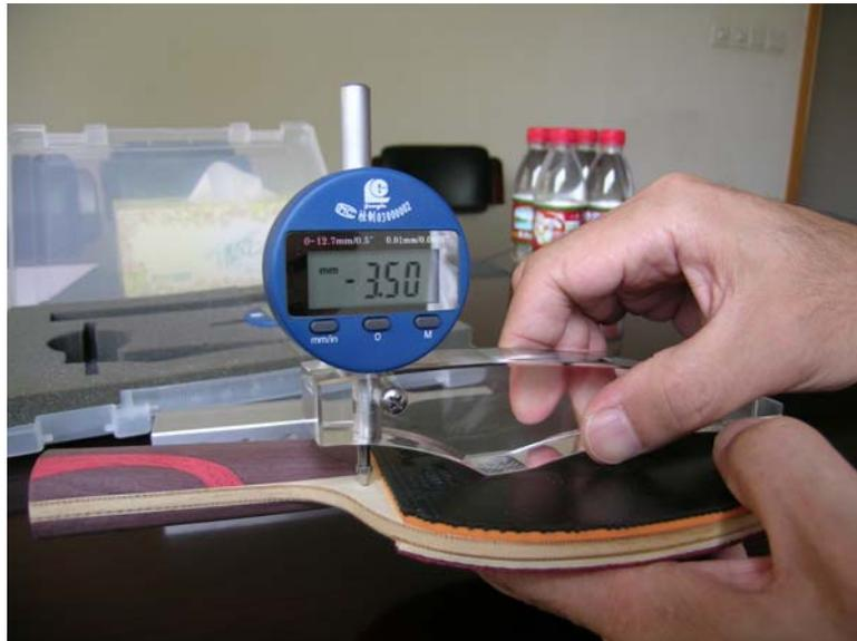
The layers in a racket must be continuous and of even thickness. Powdering, a glue pocket or zones made of different sponges under the same pimped rubber are not acceptable. Powder particles may be transferred to the ball and change the friction of opponent's rubber; differently structured sponge-layers under the top sheet give unpredictable effects. More glue may increase the speed and the spinning ability of (part of) the racket.
